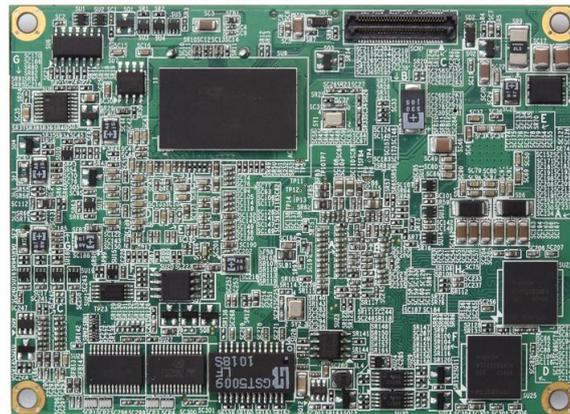
The PICO822 is a Pico-ITX board with Intel® Atom™ single core E620T/E680T and PCH EG20T chipset that delivers outstanding system performance through high-bandwidth interfaces, multiple I/O functions for interactive applications and various embedded computing solutions.
